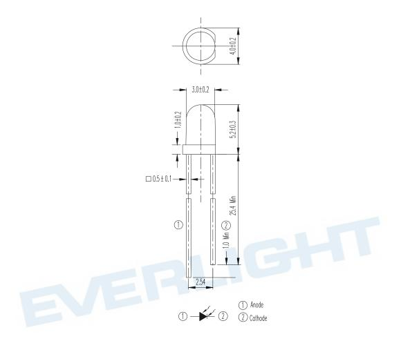
Note: Tolerances unless dimensions ±0.25mm
