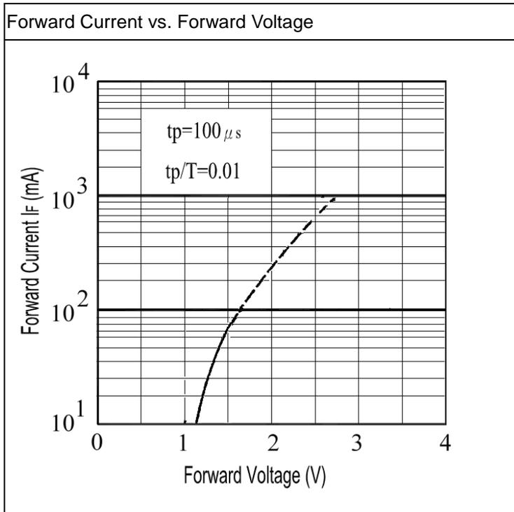
Typical Electrical/Optical/Characteristics Curves for PT
