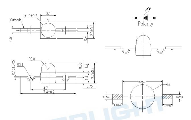
Note: The tolerances unless mentioned are ±0.1, unit=mm.
