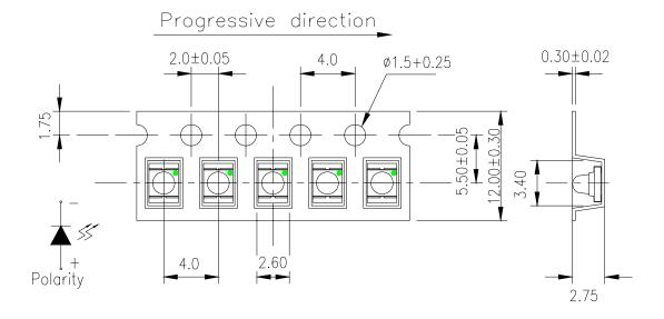
**Note:** The tolerances unless mentioned is  $\pm 0.1$ mm, Unit = mm
