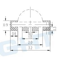
For Reflow Soldering
